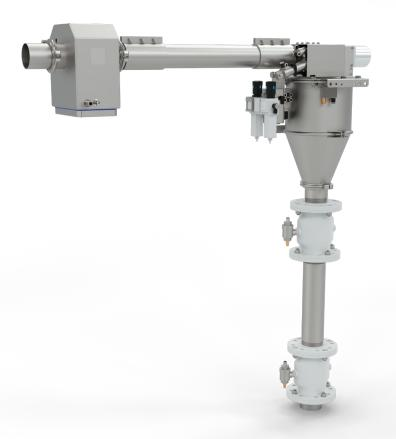
The **P-TRON 07 GM** separators are available in nominal diameters of up to 200 mm. This makes them ideal for use in silo feeders or for feeds to bagging systems. They can be used for both the pressure and vacuum conveying of powders or granulates. Contaminated material is discharged through lock valves without loss of pressure. The detection units used are optimally shielded against environmental disturbances and are also very easy to integrate into existing pipeline systems.
