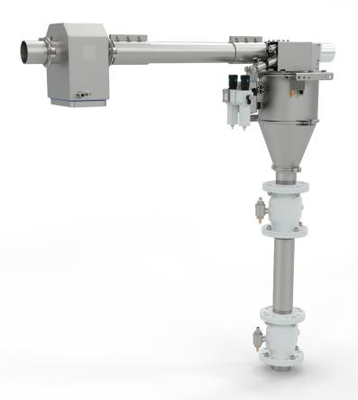
The **P-TRON 07 GM** separators are available in nominal diameters of up to 200 mm. This makes them ideal for use in silo feeders or for feeds to bagging systems. They can be used for both the pressure and vacuum conveying of powders. Contaminated material is discharged through lock valves without loss of pressure. The detection units used are optimally shielded against environmental disturbances and are also very easy to integrate into existing pipeline systems.
