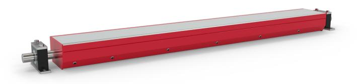
If exact spatial resolution of the impurity with respect to the width of the material web is not necessary, as is often the case in calander protection, a **METRON 05 PR** is sufficient. This plate metal detector is equipped with the AMD 05 and can therefore deliver a high degree of reliability and detection accuracy, especially for strips of up to 4,000 mm.
